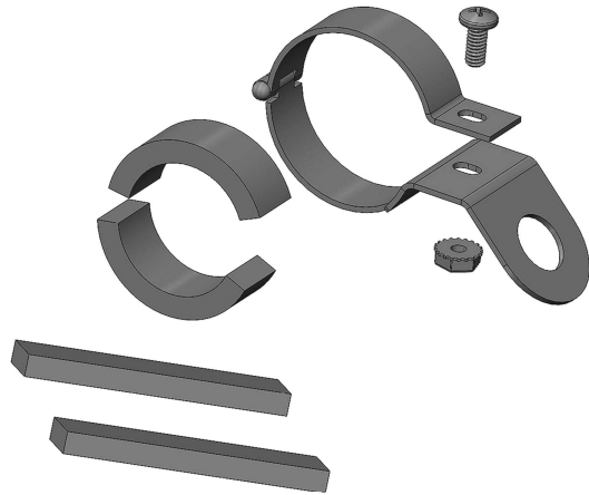
14-0083 Universal Bracket Shown with HDWR 130 hardware. Kit includes, screw, keep nut and hard rubber inserts to accommodate various diameters of mounting locations
